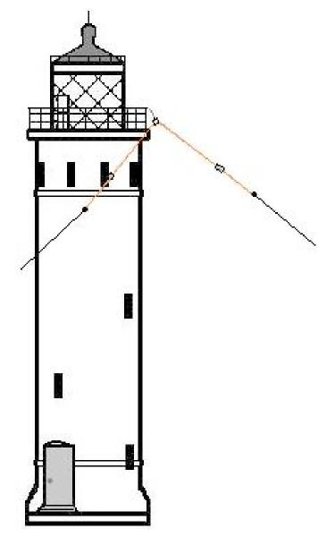
Lighthouses make great antenna masts. In this inverted "V" positioning, the dipole's usual signal characteristics, or radiation pattern, changes from what is usually a directional signal pattern to more of an omnidirectional antenna which allows for a greater range of contacts in various directions from the antenna.
