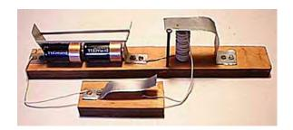
We built simple telegraph keys and sounders from scrap materials, not too different than the one shown in this picture. And while at the jamboree, hooked them up to aerial wires that had been strung between different camps and we were able to use our devices to send and receive messages in, albeit very slow, code with the other packs. This was a great introduction to what would eventually become a career in digital communications, and a dear hobby.
