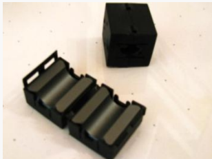
"No Mix Marked" split bead ferrite chokes (and these were sold at a ham radio store!) PHOTO: AI6DF
