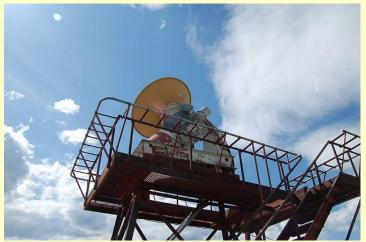
One of the two 10.7cm solar flux monitoring telescopes at the Dominion Radio Astrophysical Observatory in Penticon, BC. These telescopes provide the daily Solar Flux Index. PHOTO: JASON NISHIYAMA
