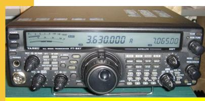
The Yaesu FT-847 multi-band transceiver, sold from 1998 through 2005, was promoted as a "satellite" radio due to its 0.1 Hz fine tuning steps for Doppler shift frequency changes; four separate antenna connections for HF, 6-meters, 2-meters, and 70-cm respectively; plus other capabilities for tracking satellites.
