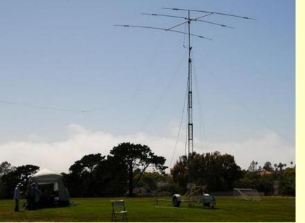
**Above:** The assembled CW antenna atop PVARC's tower trailer. PHOTO: CHRIS STOREY, KA6WNK
