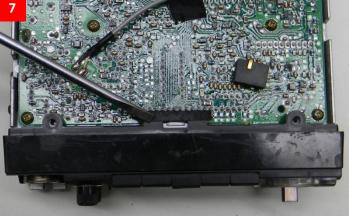
8. With that plastic cover gone, remove the three screws that hold the display electronics PC board onto the mechanical structure behind it—two on the left side (shown here) and one on the right.
