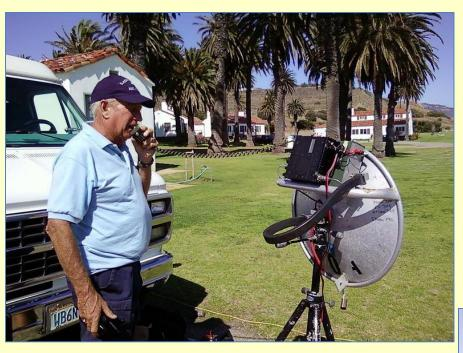
PVARC members witnessing this 110-mile contact on 10-GHz microwave were quite impressed—and with the relative simplicity of Gordon's set-up.
