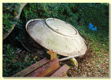
**Above**: Dish antennas 2 and 3 are made of fiberglass epoxy with an embedded metal mesh as the reflecting surface, also shown in Brian KA6UHM's backyard. The second fiberglass dish antenna is underneath the top one. Some of the angle stock that holds these dishes is shown in foreground. PHOTO: BRIAN TILLEY, KA6UHM
