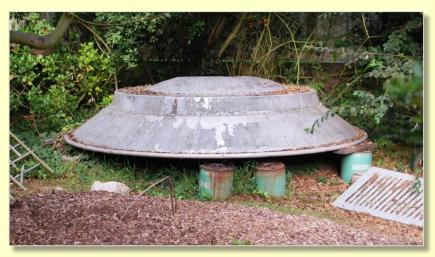
**Above**: Dish 1 is a Western Electric 3-meter diameter metal dish antenna, shown in Brian KA6UHM's backyard. PHOTO: BRIAN TILLEY, KA6UHM
