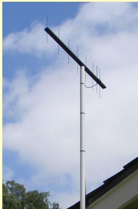
Above: 70cm inexpensive homemade Yagi built by NG6R using pine wood as the boom. Shown installed at WI6TT’s QTH in Palos Verdes Estates.
