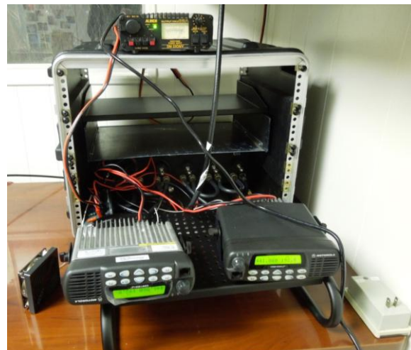
Bottom: As previously published in QRO , two of my Motorola CDM 1550 UHF radios interconnected as a 440 porta-peater for Palos Verdes Half Marathon. PHOTOS: DIANA FEINBERG, AI6DF
