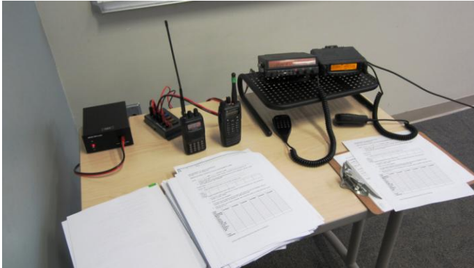
Above: AI6DF set-up at Providence Little Company of Mary Hospital--San Pedro for 2012 statewide hospital drill. Right: Close-up of Kenwood TM-742A and Yaesu FT-8800R mobile radios used at PLCM-San Pedro. Monitor stands allow mounting or positioning radios at any angle above or on the workspace. PHOTOS: AI6DF
