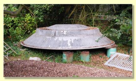
**Above**: Dish 1 is a Western Electric 3-meter diameter metal dish antenna, shown in Brian KA6UHM's backyard. PHOTO: BRIAN TILLEY, KA6UHM
