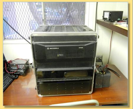
**Above:** This Motorola MTR-2000 UHF repeater loaned by Norm Thorn, K6UU, provided a hefty 50-watts for Half Marathon/10K/5K radio coverage with no worries of over-heating. Norm's repeater is rated for 100 watts continuous duty and has cavity filters plus power supply enclosed in a rugged case. PHOTO: DIANA FEINBERG, AI6DF
