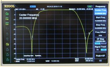
Figure 3. Triplexer 15m channel characterization test result; note deep notches at 20m and 10m, carefully tuned by adjusting wire turn spacing on appropriate inductor toroids
