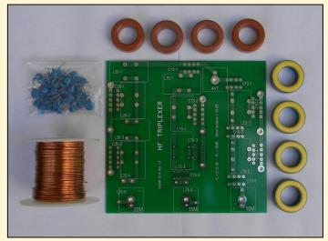
Figure 1. Parts assembled to begin construction of HF triplexer
