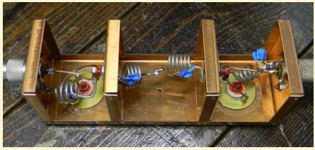
Figure 4 (above). 15m BPF constructed inside gutted TV interference LPF; each triplexer leg (10m, 15m and 20m) will have its own uniquely configured companion BPF. Figure 5 (below). 15m BPF characterization test result; note deep notches at 17m and 12m; also note >20dB isolation at 20m.
