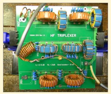
Figure 2. Fully assembled triplexer PCB undergoing 15m channel inductor tuning and characterization testing
