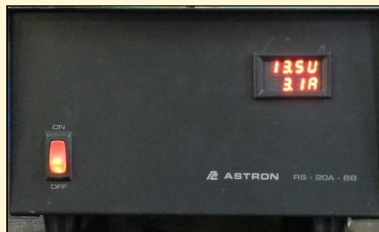
Figure 6. Astron RS-20A DC power supply before and after installation of digital voltage/current readout display; change in shading and clarity due to different lighting conditions.
