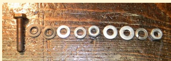
Figure 2: Order of hardware removal from negative voltage terminal
