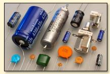
Figure 2: Examples of capacitors
