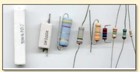
Figure 1: Examples of resistors
