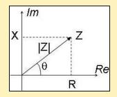
Resistance R is a real number that will always be nonnegative (right half of the plane), but reactance X can be positive (inductive) or negative (capacitive). In complex mathematics, this Cartesian coordinate frame is called the "complex plane." We can see that the magnitude of impedance (generally written as |Z|) is the hypotenuse of the triangle, i.e.,  $|Z| = v(R^2 + X^2)$
