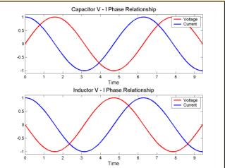
have just a couple of components or a large assortment of components in an electronic circuit, we can characterize impedance of that circuit by a "special" addition of a resistive element and a reactive element. Mathematically, we can say that Z = R + jX, Continued on next page
