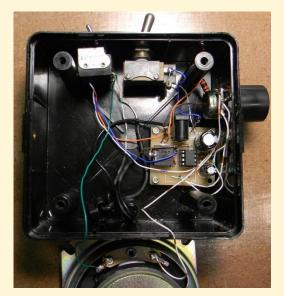
Figure 6. Audio amplifier kit assembled and installed inside another 4" comm. speaker cabinet. Also shown are the potentiometer for volume control and two external switches that control DC power on/off, powered vs. unpowered operation and amplifier hi/lo gain settings.
