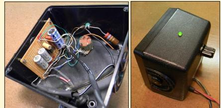
Figure 4. Audio amplifier components assembled inside the 4" speaker cabinet. DC power is brought in near the same hole in the bottom rear of the enclosure as the original speaker cable. The finished result is shown on the right.
