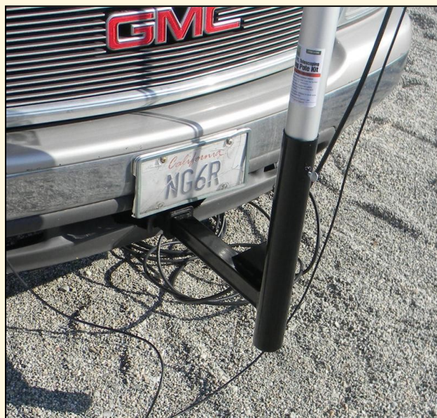
Figure 1. The “inverted V” 80m dipole is temporarily deployed for testing using a 24' mast secured using a front-vehicle-installed trailer hitch. Despite appearances, the antenna is clear of the trees. The mast is bent due to the ~100 degree azimuth angle between dipole legs.
