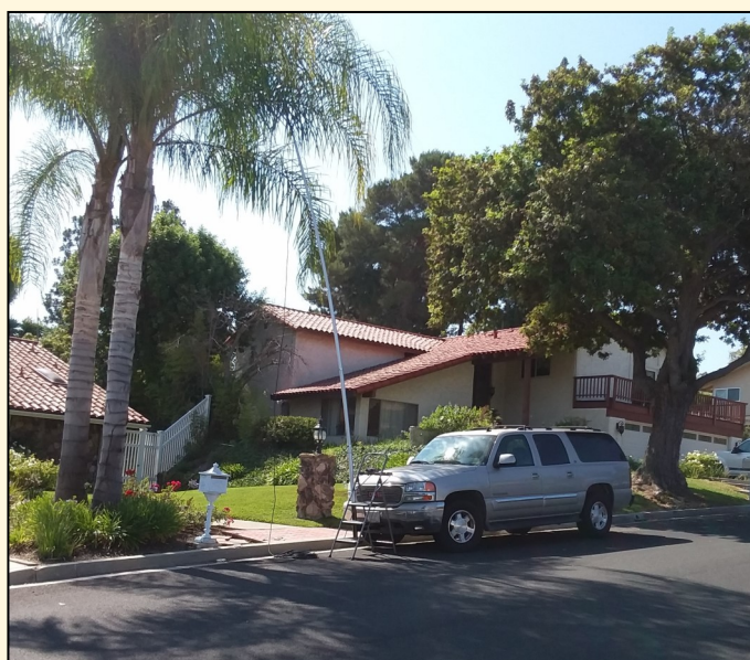
Figure 1. The “inverted V” 80m dipole is temporarily deployed for testing using a 24' mast secured using a front-vehicle-installed trailer hitch. Despite appearances, the antenna is clear of the trees. The mast is bent due to the ~100 degree azimuth angle between dipole legs.
