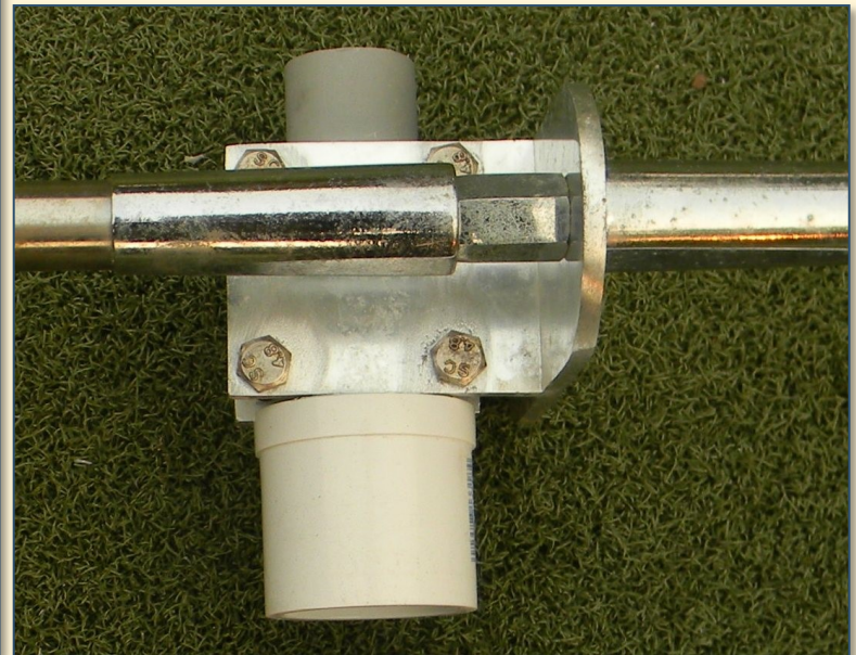
Figure 3. (left) Standard unmodified MFJ-2299 dipole (with PVC adaptor section) is used as the driven element for the Yagi.
