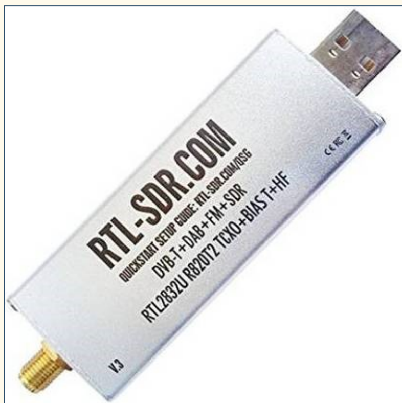
Figure 1. Stock photo of the RTL2832U R820T2 Version 3 dongle, one of the cheapest and best SDR dongles currently available. The one discussed here was purchased through Amazon.com, but they are also available from other online sources. The dongle has a USB-A connection on one end and an SMA-F antenna connection on the other end. An adaptor from SMA to SO-239, as shown, may be required for your existing indoor (or preferably outdoor) antenna(s), depending on band.
