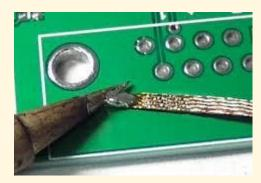
**Figure 3.** (left) Roll of fine-mesh copper braid, used to "wick" away melted solder; (center) Small container of rosin soldering flux into which the tip of the copper braid is dipped prior to each wicking attempt (very important!); (right) Hot soldering iron and braid tip are simultaneously placed onto the solder ball that is to be removed; note the flux that has soaked into the braid a few millimeters up from the tip of the braid.
