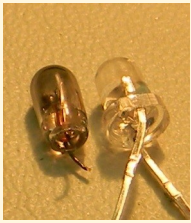
Figure 5. (1) Burned out "grain of wheat" incandescent bulb (0.115" diameter) vs. replacement LED; (2) Blue/purple LEDs installed as backlighting in author's TM-321A transceiver; (3) DIY powered speaker with green LED power-on indicator; (4) Pair of white LEDs adapted for meter display lighting in author's Tokyo Hy-Power HL-1.5KFX HF amplifier
