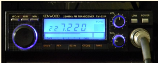
Figure 5. (1) Burned out "grain of wheat" incandescent bulb (0.115" diameter) vs. replacement LED; (2) Blue/purple LEDs installed as backlighting in author's TM-321A transceiver; (3) DIY powered speaker with green LED power-on indicator; (4) Pair of white LEDs adapted for meter display lighting in author's Tokyo Hy-Power HL-1.5KFX HF amplifier
