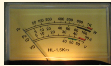
Figure 5. (1) Burned out "grain of wheat" incandescent bulb (0.115" diameter) vs. replacement LED; (2) Blue/purple LEDs installed as backlighting in author's TM-321A transceiver; (3) DIY powered speaker with green LED power-on indicator; (4) Pair of white LEDs adapted for meter display lighting in author's Tokyo Hy-Power HL-1.5KFX HF amplifier
