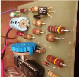
Figure 3. Close-up of Q1 2N3906 over-voltage protection circuit showing one of two base bias resistors (middle right in the photo) that readily separated from the PCB upon gentle prying; it had not been securely soldered to the PCB but the disconnect was hidden inside the through hole; the part was subsequently re-soldered as part of the repair. Note at bottom of this photo the newly installed IC socket with a new LM723 plugged into it. PHOTO: JERRY KENDRICK, NG6R
