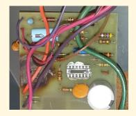
**Figure 1.** (left) Voltage regulator board with 14-pin LM723 integrated circuit shown prior to its removal; (middle) Solder side of IC prior to solder removal using flux-infused copper braid wicking technique; (right) Component side of board after installing IC socket for ease in replacing IC should it fail in the future. Note in left and right panels an area of PCB discoloration from overheating of (now removed) TIP29 driver transistor and heat sink. PHOTOS: JERRY KENDRICK, NG6R
