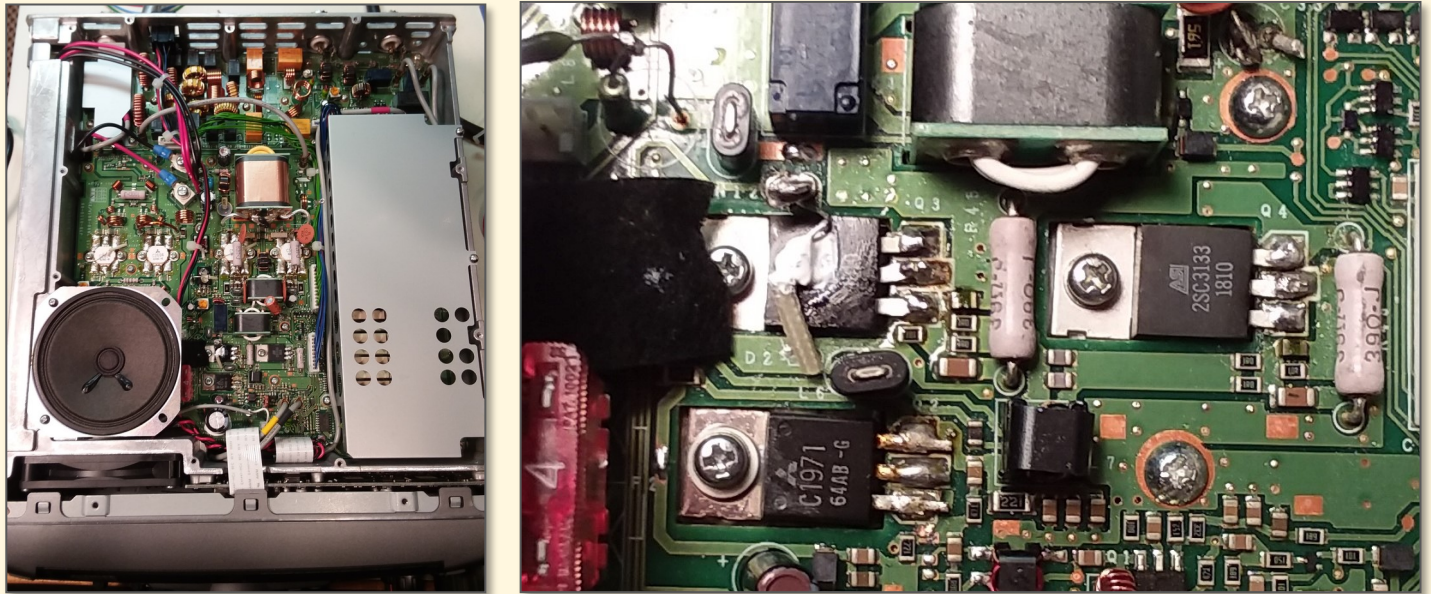
Figure 7. The two 2SC3133 equivalent replacement transistors have been installed in place of the removed 2SC1972 transistors; the temperature compensation diode was re-secured atop one of the power transistors. PHOTO: JERRY KENDRICK, NG6R
