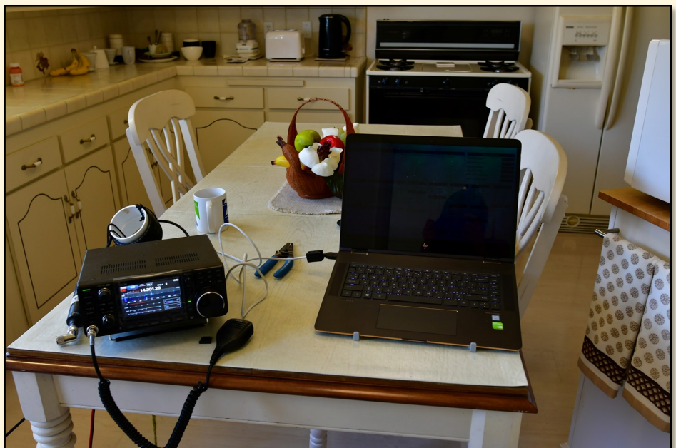
Above: 2020 Field Day operations from the kitchen table as a 1-E station using a Bioenno 40-Ah battery on the floor and PC on its internal battery. This kitchen appears somewhat dark because all AC-powered lights were off during radio operation to simulate outage conditions. PHOTO: DIANA FEINBERG, AI6DF
