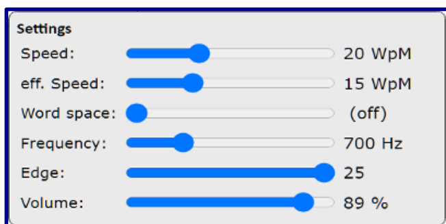
Figure 3. The Settings window for fine-tuning the nature of the Morse code audio being sent. ► Next page...
