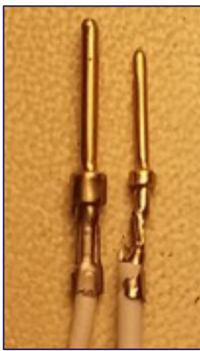
Figure 2. Side by side comparison of push-through pins for two user-configurable male connectors: DB9 on the left, HD15 on the right
