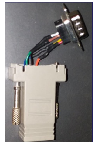
Figure 3. DB9-to-RJ45 adapter reconfigured by snipping off and discarding all DB9 pins and then soldering onto pin wires 1, 2, 3 and 5 (blue, orange, black, green, respectively) the harvested unused (and smaller diameter) pins (4, 6, 7 and 8) from earlier configured HD15 adapters
