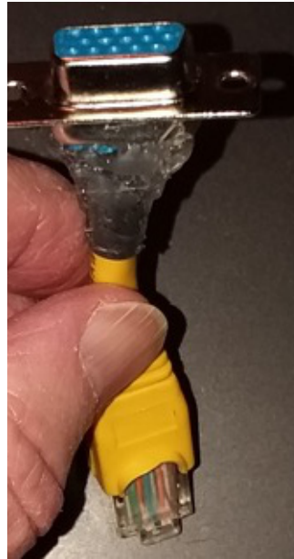
Figure 6. (left) Test jig used to confirm construction accuracy and verify no wiring errors in both compact adapters and soldered cable connector adapters.
