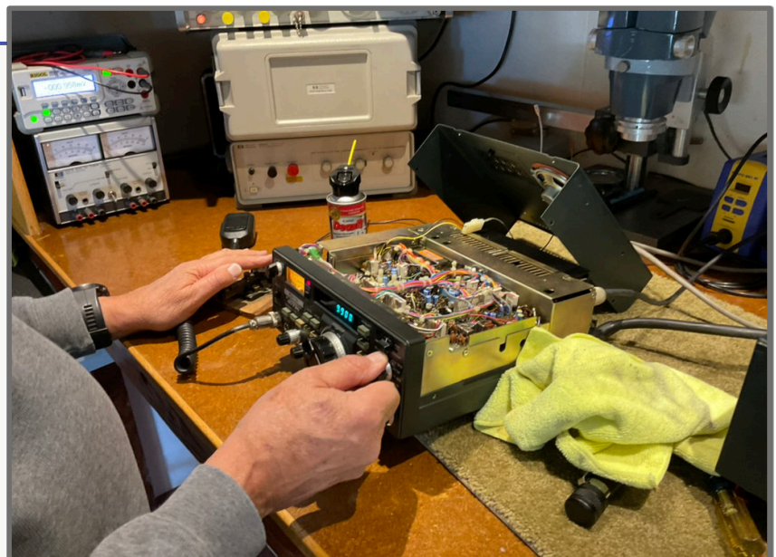
Above: Our member Gary Lopes WA6MEM signal tests a donated ICOM HF transceiver prepared for sale to benefit the ARRL's ARES-LAX program. PHOTO: DIANA FEINBERG, AI6DF
