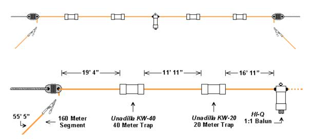
\*For 160 Meter Band use, the antenna is lowered via a pulley system so the 55' 5" 160 Meter segments can be alligator clipped to the ends of the dipole
